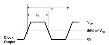
Figure 3. ER =  $(0.6 \text{ x V}_{DD})/t3$ , EF =  $(0.6 \text{ x V}_{DD})/t4$
