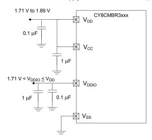
\*SUPPLY\_LOW\_POWER bit in DEVICE\_CFG3 register should be set to 1 to operate device at 1.8V ( $\pm 5\%$ )
