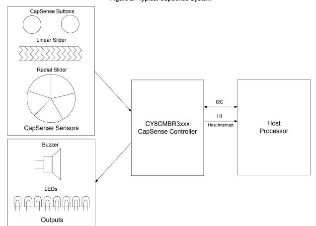
Figure 2. Typical CapSense System
