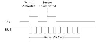
If the buzzer is not currently active, the buzzer output starts on each trigger event.
