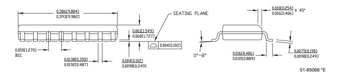
Figure 25. 8-pin SOIC (150 Mils) Package Outline
