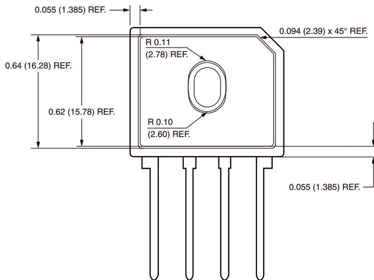
**FORMING SPECIFICATION: BU-5S** in inches (millimeters)
