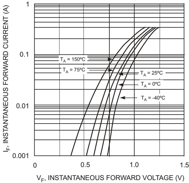
Fig. 1 Forward Characteristics
