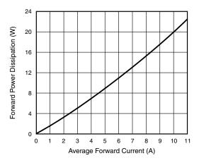
Fig. 3 - Forward Power Dissipation
