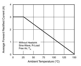
Fig. 2 - Forward Current Derating Curve
