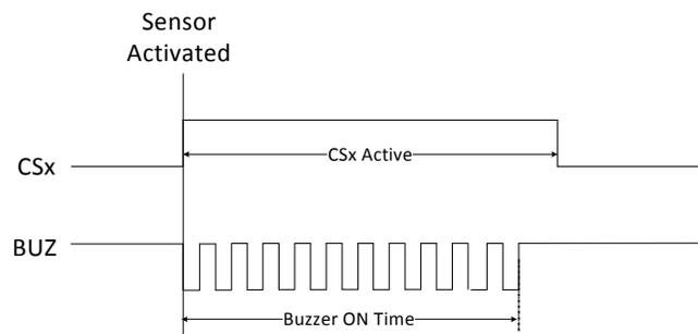
The buzzer output does not restart if multiple trigger events occur before the Buzzer ON Time elapses.
