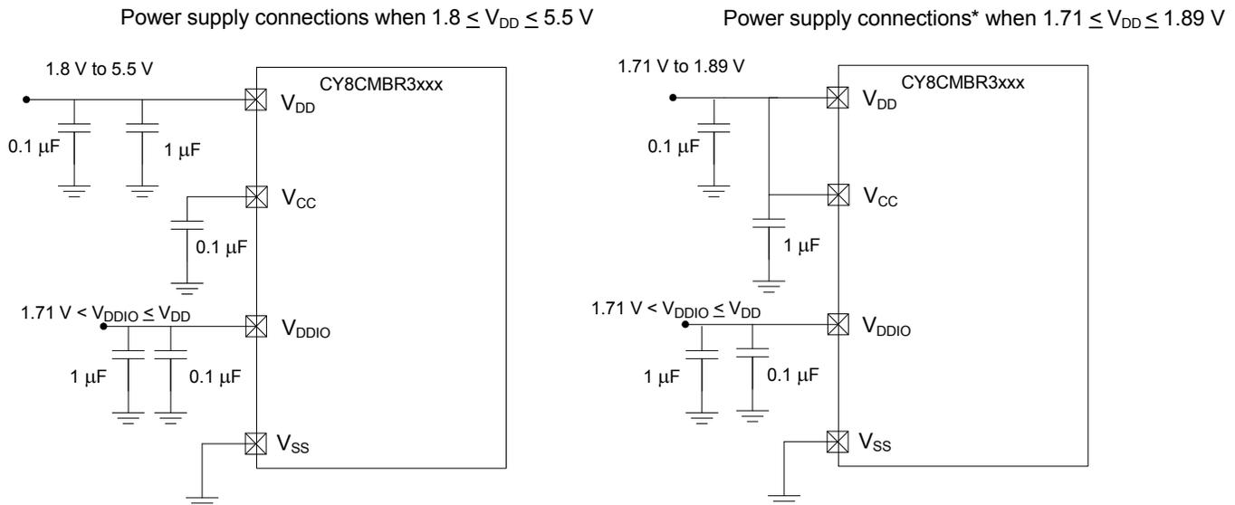
\*SUPPLY\_LOW\_POWER bit in DEVICE\_CFG3 register should be set to 1 to operate device at  $1.8\text{ V} (\pm 5\%)$
