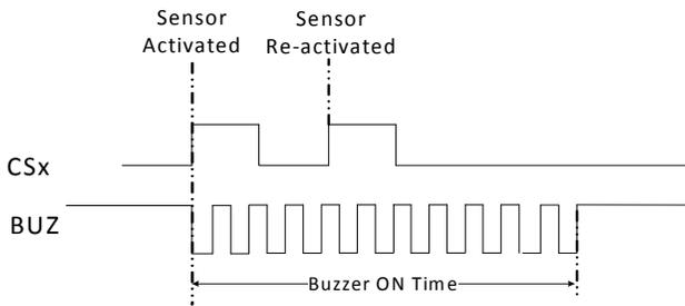
If the buzzer is not currently active, the buzzer output starts on each trigger event.
