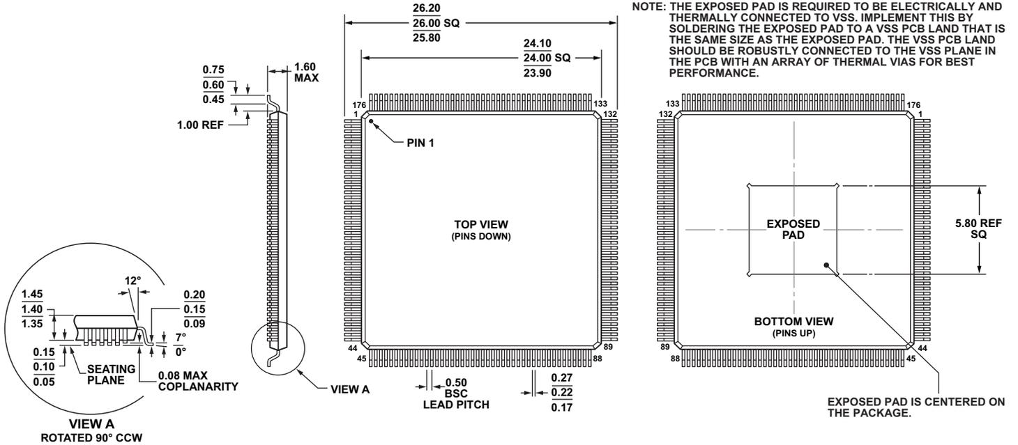
Figure 58. 176-Lead Low Profile Quad Flat Package [LQFP\_EP] (SQ-176-2)
