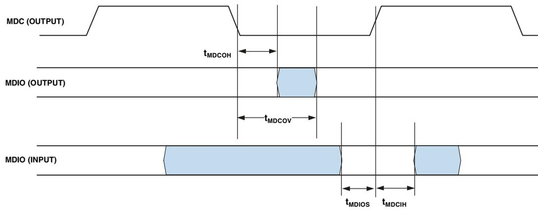
Figure 31. 10/100 Ethernet MAC Controller Timing: MII Station Management
