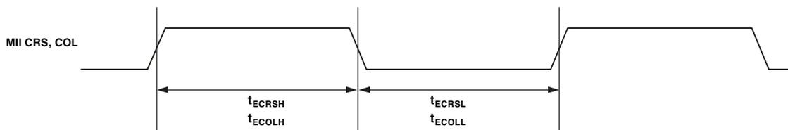
Figure 30. 10/100 Ethernet MAC Controller Timing: Asynchronous Signal
