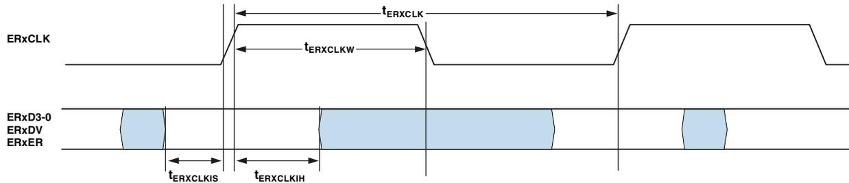
Figure 26. 10/100 Ethernet MAC Controller Timing: MII Receive Signal
