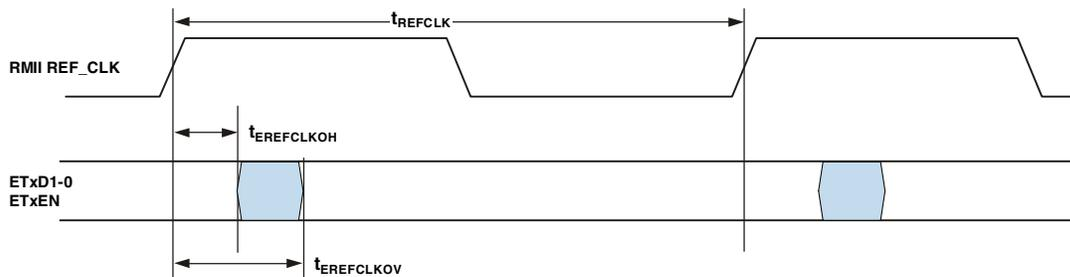
Figure 29. 10/100 Ethernet MAC Controller Timing: RMI Transmit Signal
