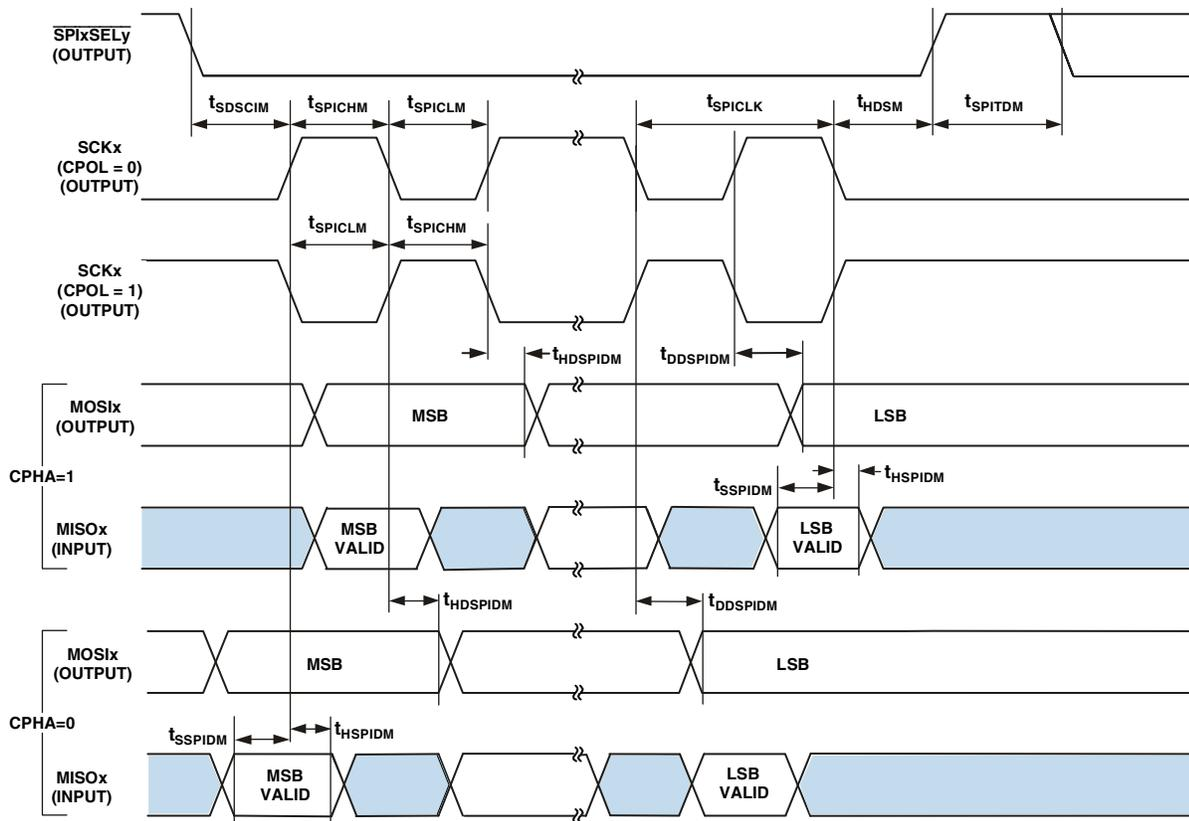
Figure 20. Serial Peripheral Interface (SPI) Port—Master Timing
