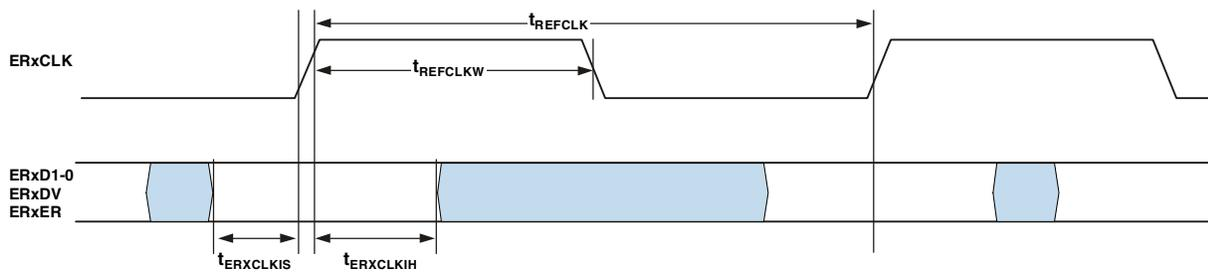
Figure 28. 10/100 Ethernet MAC Controller Timing: RMI Receive Signal
