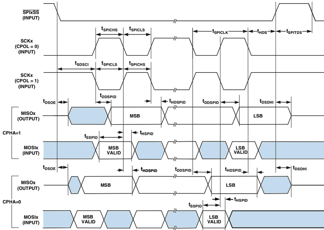
Figure 21. Serial Peripheral Interface (SPI) Port—Slave Timing
