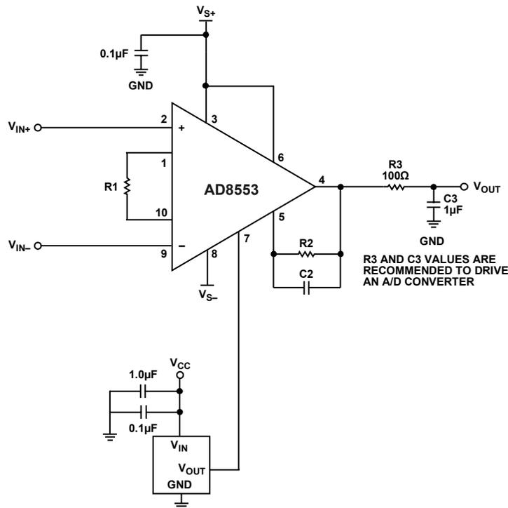
Figure 34. Dual-Supply Connection Diagram Using IC Voltage Reference
