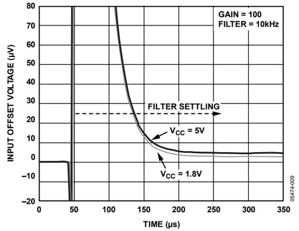
Figure 11. Input Offset Voltage vs. Turn-On Time
