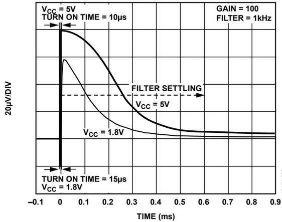
Figure 8. Input Offset Voltage vs. Turn-On Time
