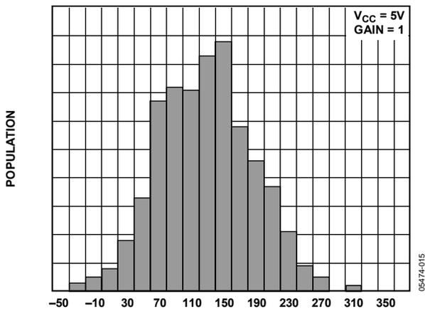
Figure 15. Input Offset Voltage ( $\mu\text{V}$ )
