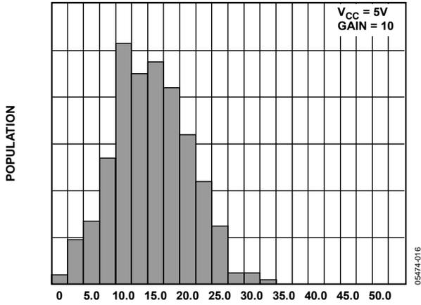
Figure 14. Input Offset Voltage ( $\mu\text{V}$ )
