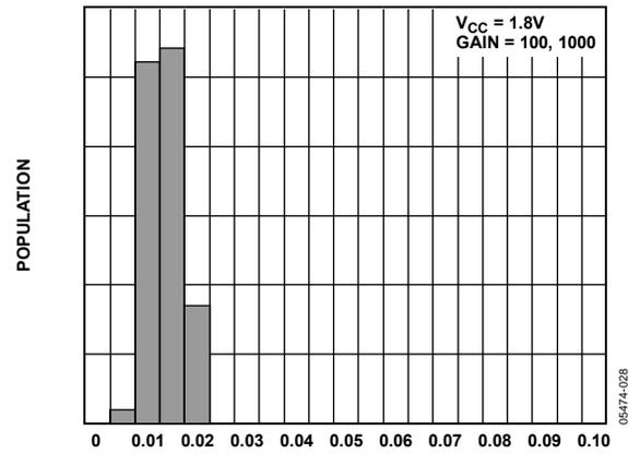
Figure 24. Input Offset Voltage Drift ( $\mu V/^\circ C$ )
