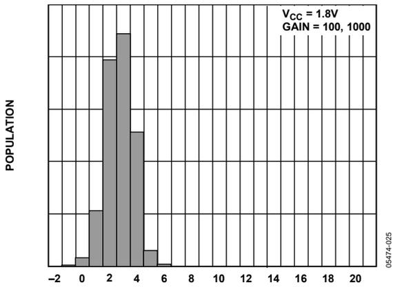
Figure 21. Input Offset Voltage ( $\mu V$ )
