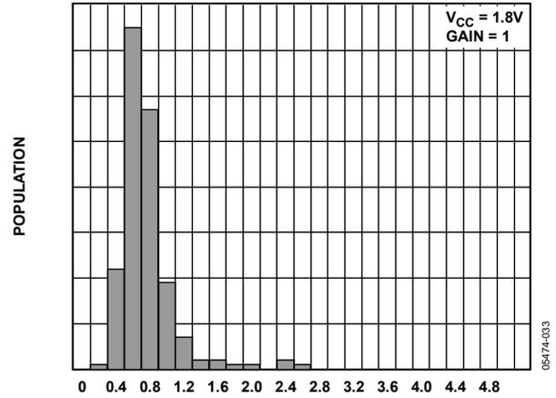
Figure 28. Input Offset Voltage Drift ( $\mu\text{V}/^\circ\text{C}$ )
