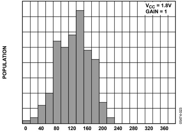
Figure 26. Input Offset Voltage ( $\mu\text{V}$ )
