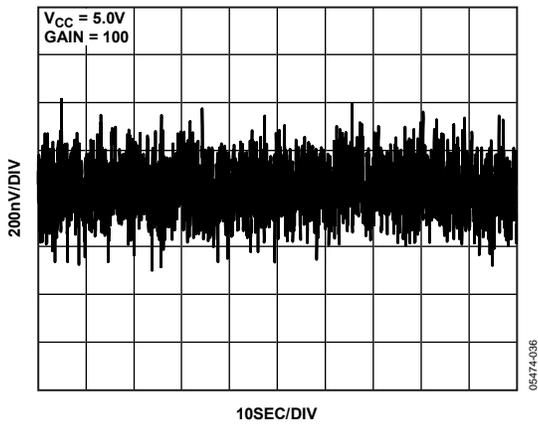
Figure 27. 0.01 Hz to 10 Hz Voltage Noise
