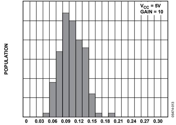
Figure 17. Input Offset Voltage Drift ( $\mu\text{V}/^\circ\text{C}$ )
