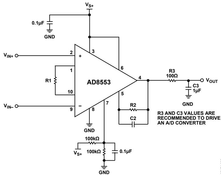
Figure 31. Single-Supply Connection Diagram Using Voltage Divider Reference
