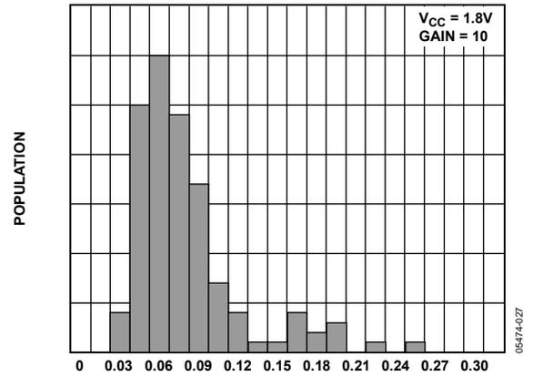
Figure 25. Input Offset Voltage Drift ( $\mu V/^\circ C$ )
