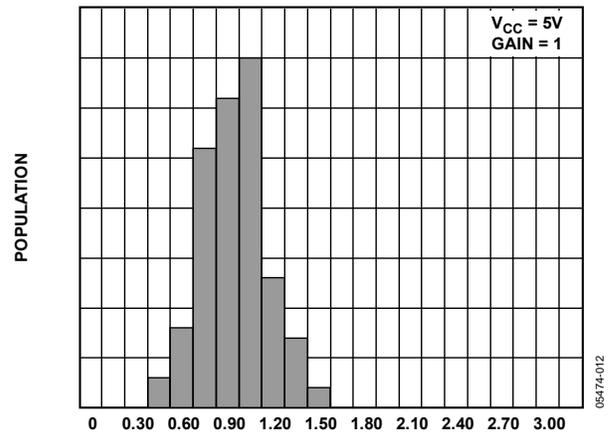
Figure 18. Input Offset Voltage Drift ( $\mu\text{V}/^\circ\text{C}$ )
