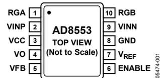
Figure 1. 10-Lead MSOP
