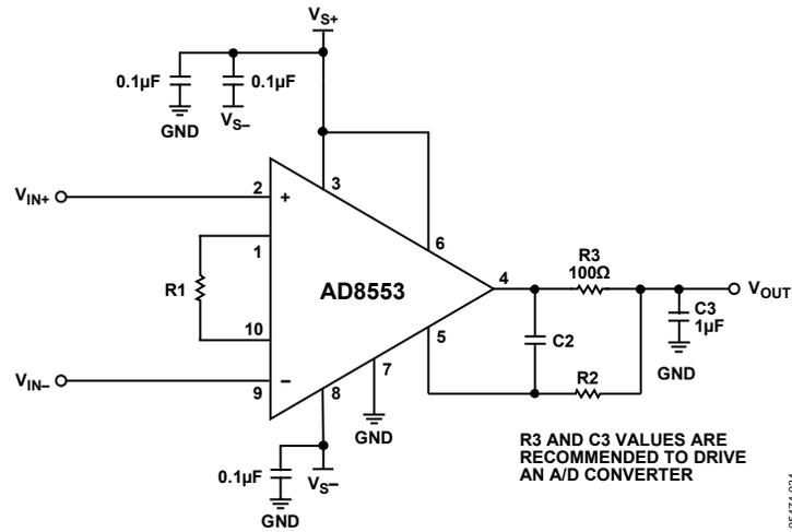
Figure 33. Dual-Supply Connection Diagram with Low Impedance Output
