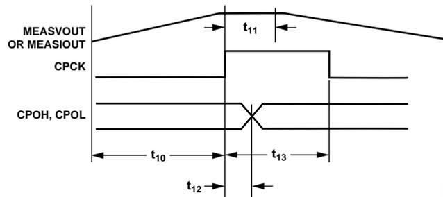
Figure 3. Comparator Timing
