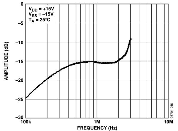
Figure 16. Force Amplifier AC PSRR, Mode 3,  $C_{COMP} = 100$  pF
