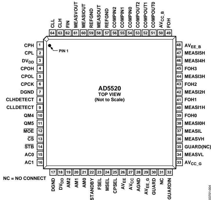
Figure 4. Pin Configuration
