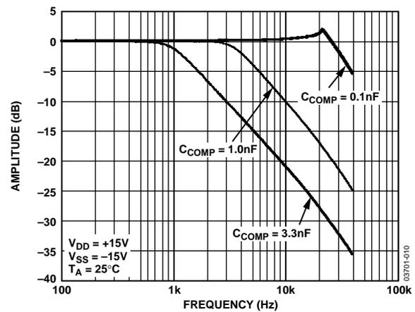
Figure 10. Force Amplifier Bandwidth, Mode 1 (40  $\mu$ A)
