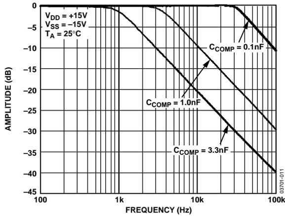
Figure 11. Force Amplifier Bandwidth, Mode 2 (400  $\mu$ A)
