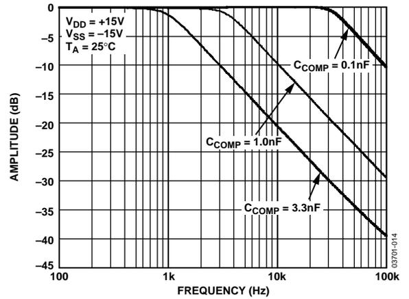
Figure 14. Force Amplifier Bandwidth, Mode 3 (4 mA)
