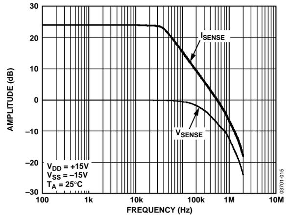
Figure 15. Voltage Sense and Current Sense Amplifier Bandwidths
