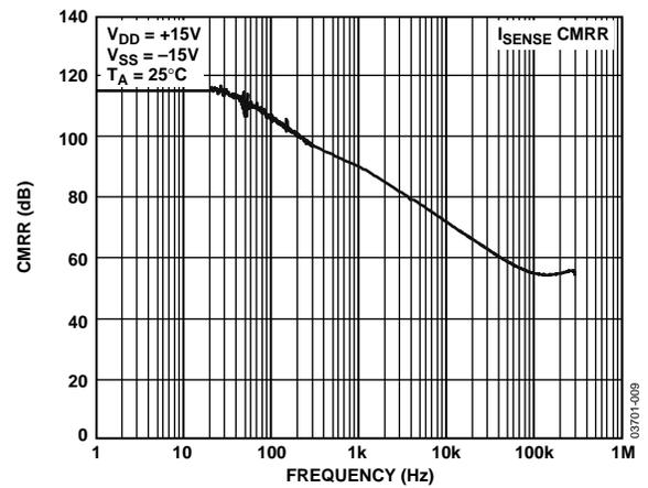
Figure 9. Current Sense Amplifier CMRR vs. Frequency
