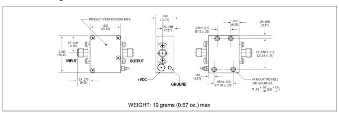
\* Dimensions are inches (millimeters) ±0.015 (0.38) unless otherwise specified.
