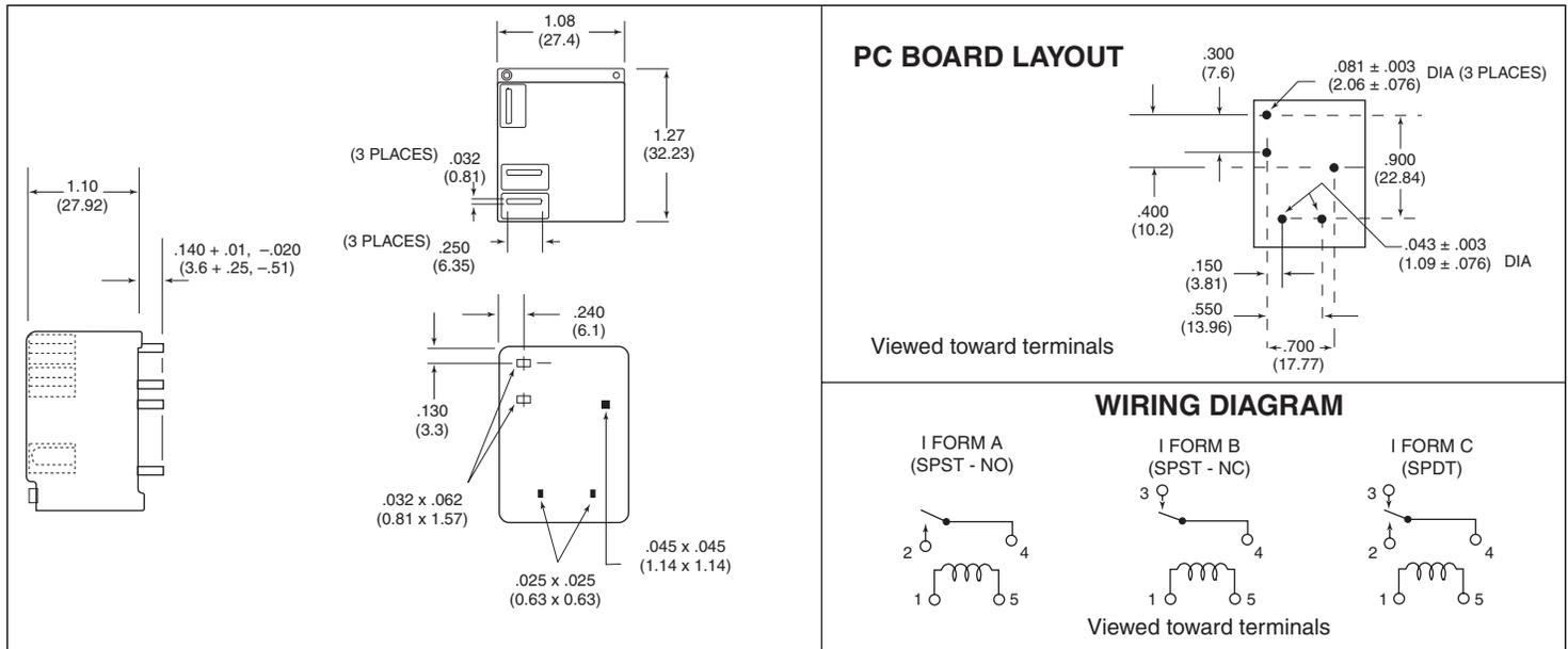
Dimensions in inches with metric equivalents in parentheses. Tolerance:  $\pm .010$ "
