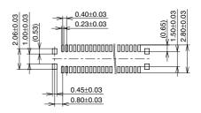
Recommended metal mask opening pattern Metal mask thickness: When 120µm
