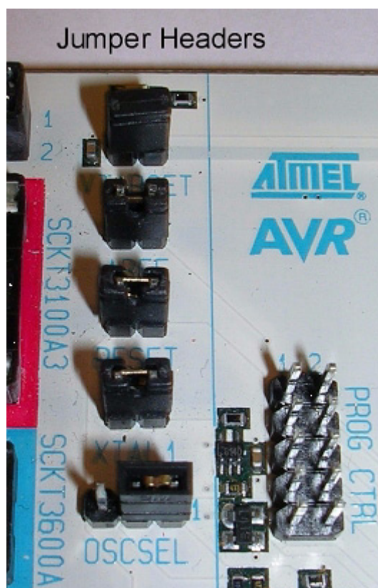
Figure 2-2. Detail of Jumper Placement on the STK500
