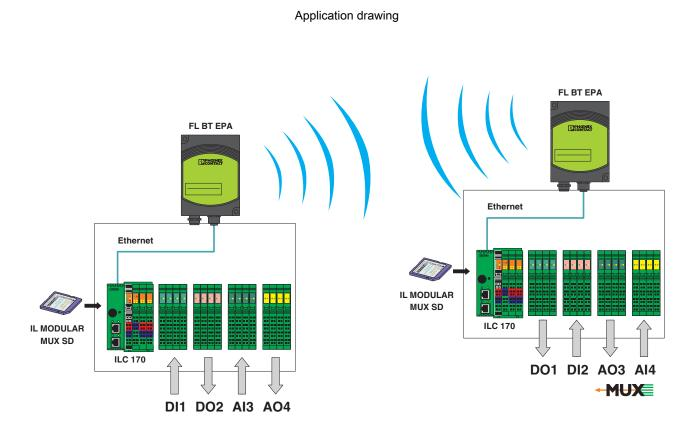
The software on the SD FLASH 512MB MODULAR MUX CompactFlash<sup>®</sup> card transforms the ILC 131 ETH and the individual input and output terminals required into a flexible field multiplexer. As a wireless connection or as a point-to-point connection in an Ethernet network.
