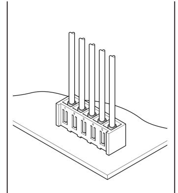
The SDN connector is a 3.96mm pitch board-in crimp style connector capable of connecting a wide variety of circuits including signal and power supply circuits. The connector features a slim, low-profile design. In addition, it has an exclusive lance construction to reduce insertion force, thus substantially improving the working efficiency in mounting the contact.
