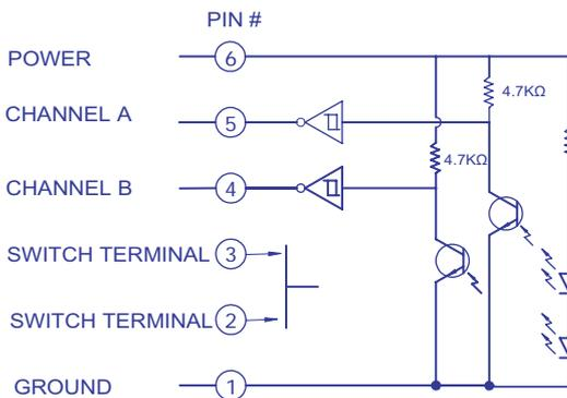
\* Schmitt trigger and pull-up resistors (4.7K $\Omega$ ) are integrated inside CTS optical encoder, so it's not necessary to have external pull-up resistors for application circuit.
