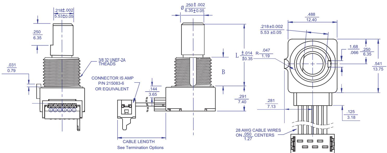
**TYPE 291V1...S** 2-Bit Encoder With Schmitt Trigger, Without Locating Lug, 0.05" Pitch Pins Formed to Rear
