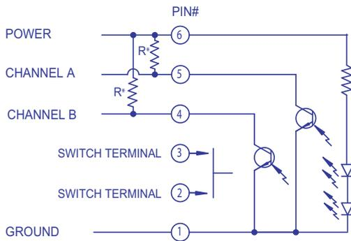
\* Require pull-up resistors (2.2K or 4.7K  $\Omega$ ) for application
