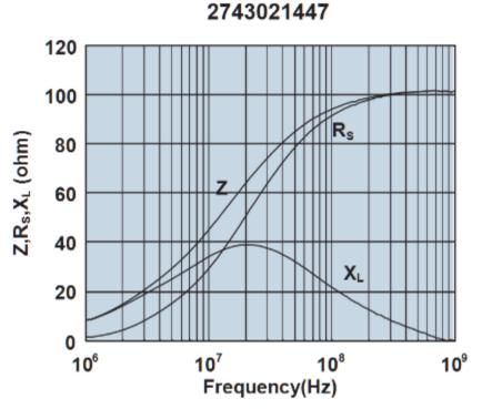
Impedance, reactance, and resistance vs. frequency.
