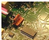
Pictured to the right is an ICE-Cube connected directly to a project PCB (the PSoCEval). ISSP can be done with the small ISSP connector. An ISSP connector is pictured to the left. See Application Notes AN 2014 and AN2026 for more information on ISSP.
