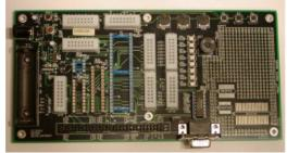
The PSoC PROTO BOARD is a complete standalone development board for evaluating and developing applications using PSoC devices. It was created to give engineers the ability to develop and test applications without creating their own custom board. It is easily configurable to schematically "look like" your end application. It allows development with any PSoC device in a DIP package.
