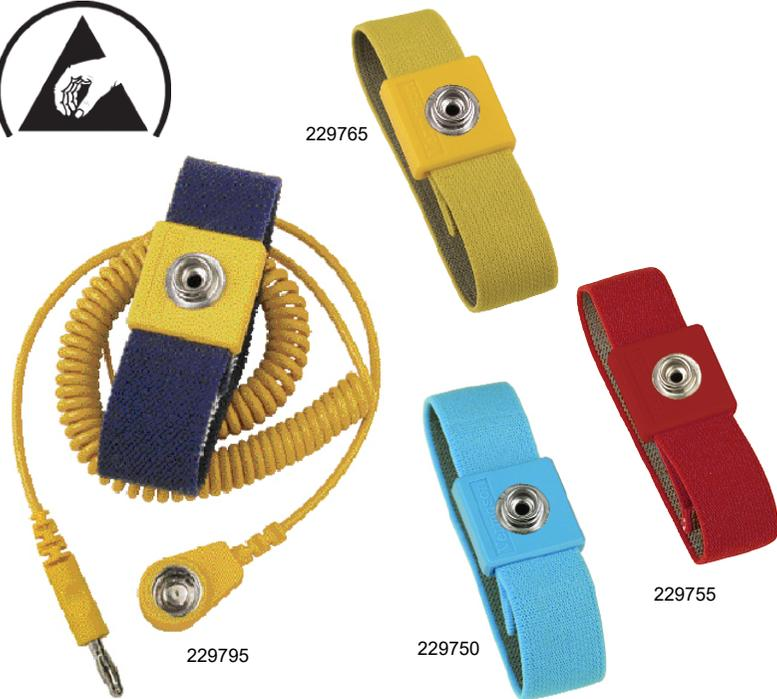
**Designed to be used with a Coiled Cord (included with Wrist Straps) with a one megohm current limiting resistor meeting the EN 61340-5-1 Personnel Grounding requirements tested per ANSI/ESD S1.1.**
