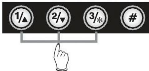
4.2. Pressing button “#” and buttons “1, 2, 3”, you can store the setting temperature into fast channel knobs “1, 2, 3”.
