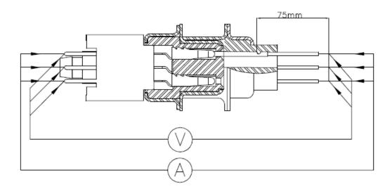
Termination resistance shall be found by subtracting the resistance of 75mm long wire from the Measured value.
