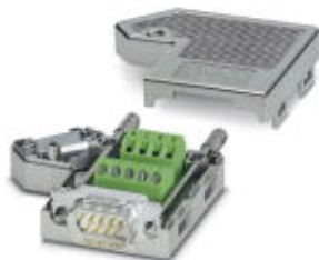
D-SUB connector, 9-pos., male connector, one cable entry < 35°, universal type for all systems, pin assignment: 1, 2, 3, 4, 5, 6, 7, 8, 9 to screw connection terminal block
