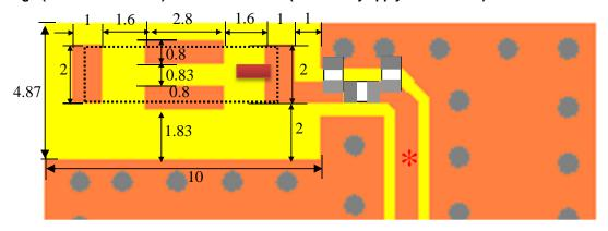
IMPORTANT! Matching circuit and component values will be different on your PCB, this will depend on PCB layout and shape, encasment, etc
