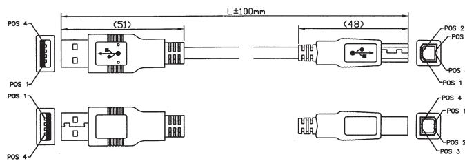
2431 01 UL2725 AWG28 x 1P + AWG24 x 2C + Al-Foil + Drain + Braid
