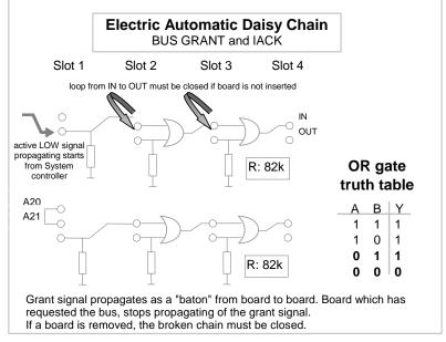
Automatic Daisy Chain (ADC), realized by a special connector with mechanical switches inside. This option is available on request.
