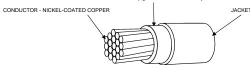
JACKET - RADIATION-CROSSLINKED, MODIFIED ETFE
