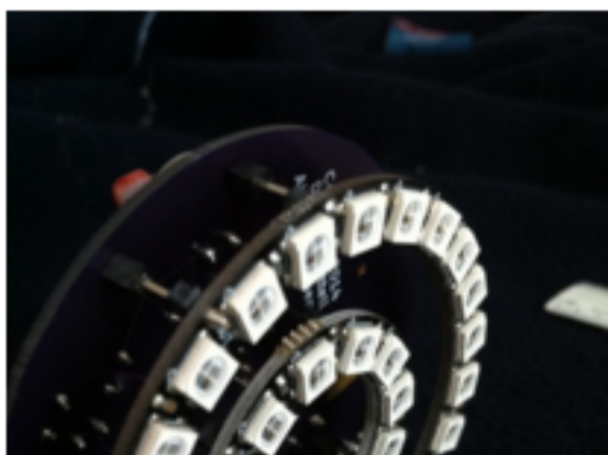
Madison's NeoClock - A PIC + KiCAD + NeoPixel adventure A NeoPixel desk clock you may only have to set once.
