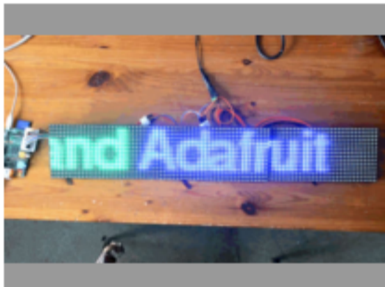
16x32 RGB Display with Raspberry Pi - part 2 Daisy-chain three 16x32 LED Displays with a Raspberry Pi
