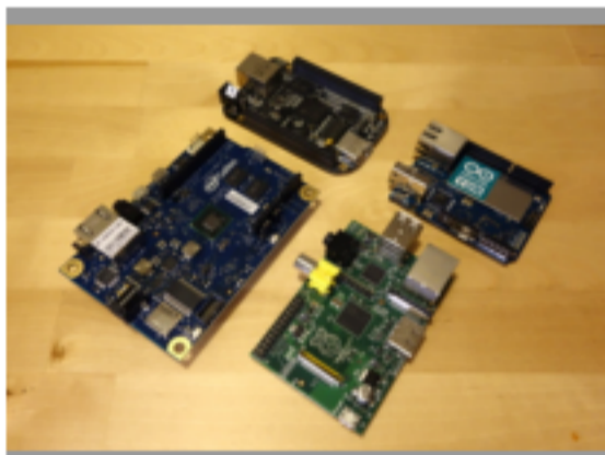
Embedded Linux Board Comparison Raspberry Pi, Beaglebone Black, Arduino Yun, and Intel Galileo--which one is right for you?
