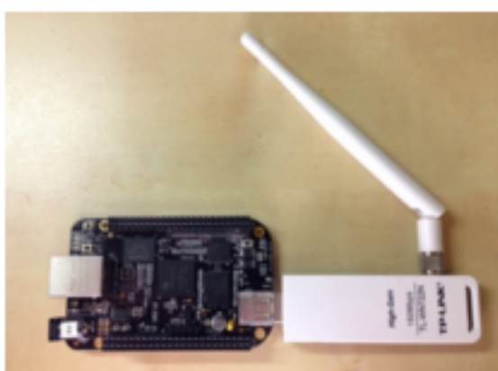
Setting up WiFi with BeagleBone Black Use a USB WiFi adapter to get your BeagleBone Black on the Internet!
