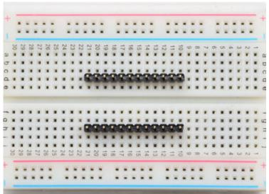
Cut the strip to length if necessary. It will be easier to solder if you insert it into a breadboard - **long pins down**
