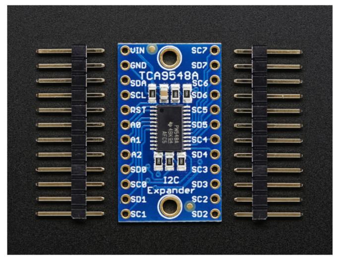
Finally, a way to get up to 8 same-address I2C devices hooked up to one microcontroller - this multiplexer acts as a gatekeeper, shuttling the commands to the selected set of I2C pins with your command.
