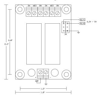
Note: The two pins at the J4 (pins 5/6) label are both ground pins, while the pins labeled RLY1 and RLY2 (pins 1/2) are the signal/control pins. Pins 3 and 4 are no connected but allowed you to connect a powered servo cable without a conflict with the servo supply.
