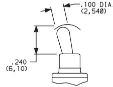
Material: Nylon 4/6 (UL 94V-0), black standard. Static resistance: 9,000 V DC min. @ sea level, actuator to terminals. Not available with F1 conductive bushing option. Not UL approved.
