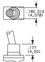
**NOTE:** ESD protection depends on proper grounding of switch support bracket. F1 conductive bushing option is impregnated with carbon fibers; dissipates electrostatic discharge (ESD) up to 20,000 V from actuator to ground.
