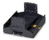
DIN rail housing for use in distribution boards in accordance with DIN 43880, Lower housing part with base latch, width: 107.6 mm, height: 89.7 mm, depth: 48.9 mm, cross connection: DIN rail connector (optional), number of positions cross connector: 16, color: black (9005)
