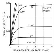
Fig.1 Typical output characteristics
