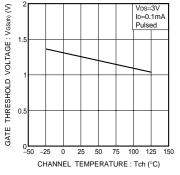
Fig.3 Gate threshold voltage vs. channel temperature
