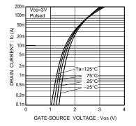
Fig.2 Typical transfer characteristics
