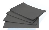
Q-ZORB PN 2242, RFSW-S-125-FR-PSA is a flexible elastomeric magnetic absorbing material. The material is designed to perform well for surface current attenuation. It can be used to lower the Q of cavities and reduce EMI. It is easily bonded using contact adhesives or it can be supplied with a pressure sensitive acrylic adhesive (PSA).
