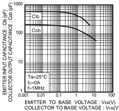
Fig.5 Collector Output Capacitance vs. Collector-Base Voltage
