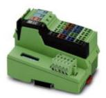
Inline, Bus coupler, DeviceNet™, TWIN COMBICON, Digital inputs: 8, 24 V DC, Connection method: 3-conductor, Digital outputs: 4, 24 V DC, 500 mA, Connection method: 3-conductor, Transmission speed in the local bus 500 kbps / 2 Mbps, Degree of protection IP20, including Inline connectors and marking fields
