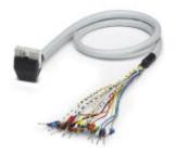
Round cable set; Connection 1: Single wires (50-position) (The wires are marked and fitted with ferrules.); Connection 2: IDC/FLK socket strip (1x 50-position, 90 °-Out put); Cable length: 2 m
