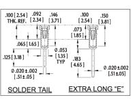
"A" = NO. OF PINS PER ROW x 0.100 [2.54] "B"= (NO. OF PINS PER ROW -1) x 0.100 [2.54]
