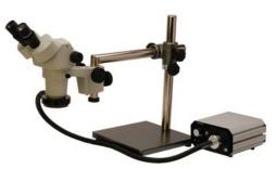
Binocular Scope on Single Arm Boom Stand with Fiber Optic Illumination
