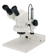
Large stage to accommodate large parts. A long life and low temperature 9W fluorescent lamp is used for the built-in incident light. Magnification: 10x & 30x
