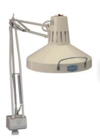
Features a 9 1/2" shade with a 22-watt fluorescent and a 60-watt incandescent bulb. A 3-way switch permits selection of fluorescent or incandescent or both. A 42" adjustable spring balanced arm with tension control allows you to position the lamp exactly where you require. Ivory color. Comes with a c-mounting clamp and a 5-foot power cord. Operates at 115V-AC.
