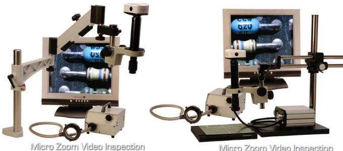
Micro Zoom Video Inspection System on Articulating Arm 26700-102-15 Micro Zoom Video Inspection System on Boom Stand 2700-102-10
