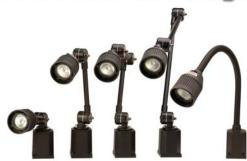
Excellent for all types of applications requiring high intensity illumination, such as manufacturing, assembly, and inspection. Round tube arms are vibration resistant but can be adjusted to provide the lighting angle you require (Also available with a flex arm). Lamp Head can be moved in up and down direction. 20 Watt Halogen bulb included. Can accept up to 50 watt bulb. C-Clamp is included. Optional Magnetic Base also available. Industrial Grade Quality. 1-year warranty (excludes bulb).
