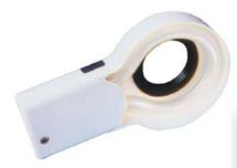
Aven fluorescent ring lights are designed for applications requiring a high quality illuminator. Provides 360° shadow free illumination. Our reflector housing is cast from high quality aluminum alloy (except for model 26200B-201) for durable and cool operation. Features a 17 Watt lamp with 5000 hours of lamp life. (5600 kelvin). Color: Putty. Operates at 115VAC
