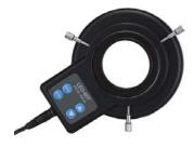
Designed to be used with standard microscopes and video lenses. Has a 7 step brightness control feature and four lighting modes, 1/4, 2/4, 3/4, and Full. Excellent for applications requiring a high degree of lighting control. Incorporates 60 Long Life LEDs that are flicker free and operate at low temperature and does not change color over time. 110V.
