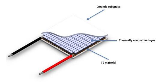
Figure 1 Cut out of a TEM device
