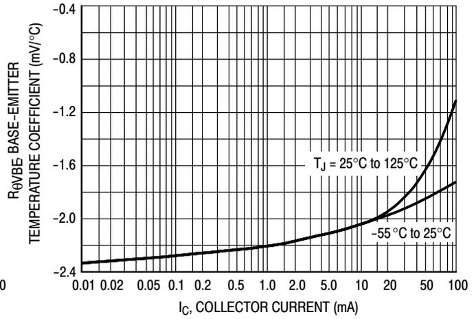
Figure 10. Temperature Coefficients
