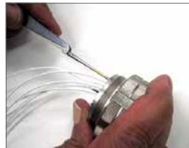
Removal of contacts with metal tool.
