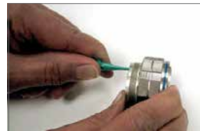
Plastic tool with contact in proper position.
