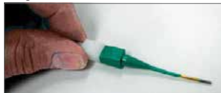
Plastic tool with contact in proper position.
