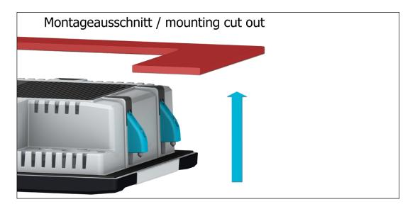
2) Then insert the device into the recess created in the described way. The tensioners will snap back.
