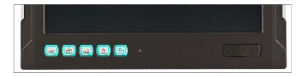
Depending on the equipment version, an operating system and a soft keyboard has previously been installed ex works. The keys on the front panel are occupied with the following functions by a specific driver in the soft keyboard:
