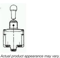
TL Series Toggle Switch, 2 pole, 2 position, Screw terminal, Locking
