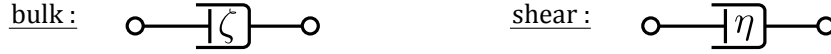
Figure 6: The bulk part (left) and the shear part (right) for a Navier-Stokes (or Newtonian) fluid. A dashpot yields a viscous stress proportional to the time derivative of the induced metric.
