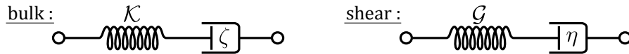
Figure 8: The bulk part (left) and the shear part (right) for a Maxwell material.
