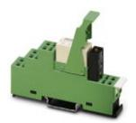
Preassembled relay modules with spring-cage connection, consisting of: Relay socket plug-in miniature power relay with power contacts, plug-in display/interference suppression module and relay retaining bracket. Input voltage: 120 V AC, contacts: 1 PDT, 10 A
