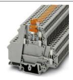
Knife disconnect terminal block, With test socket screws for insertion of test plugs, Connection type: Screw connection, Cross section: 0.2 mm² - 4 mm², AWG: 24 - 12, Nominal current: 26 A, Nominal voltage: 400 V, Length: 80 mm, Width: 6 mm, Color: gray, Assembly: NS 35/7,5, NS 35/15, NS 32
