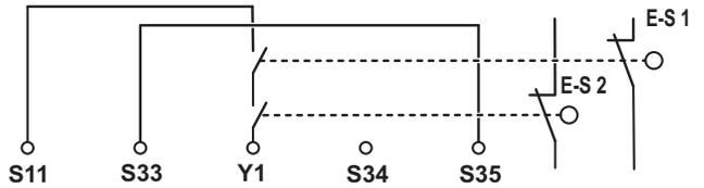
Figure 18 Automatic activation with restart inhibit in the event of mains failure (E-S1, E-S2)
