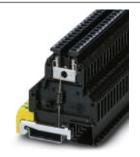
Modular terminal block with suppressor diode as surge voltage protection between clamping connector and DIN rail, separate ground connection, nominal voltage: 12 V DC, mounting on NS 35/7.5, terminal width: 6.2 mm, terminal height: 69 mm
