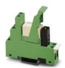
Preassembled relay modules with screw connection, consisting of: Relay socket plug-in miniature power relay with power contacts, plug-in display/interference suppression module and relay retaining bracket. Input voltage: 24 V AC, contacts: 1 PDT, 12 A
